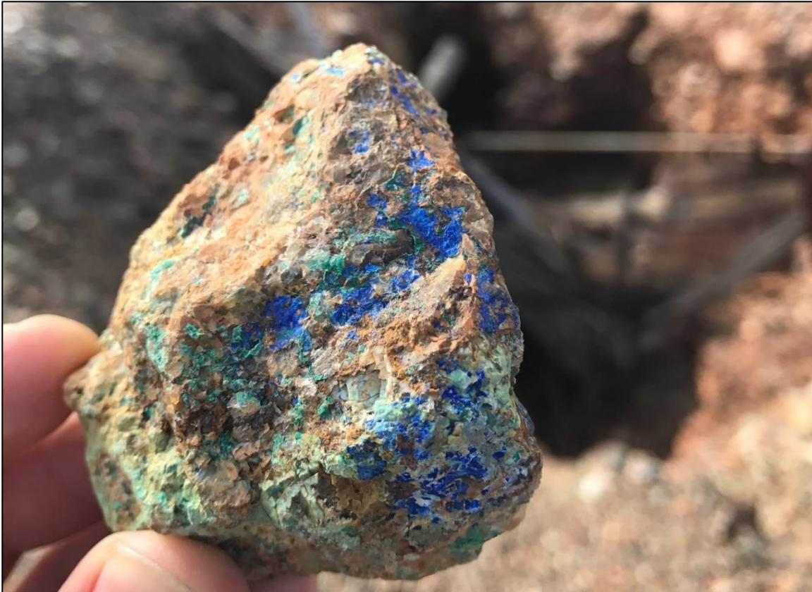
Figure 5. Malachite and azurite mineralisation from historic mine workings at Reward Copper-Gold Prospect
