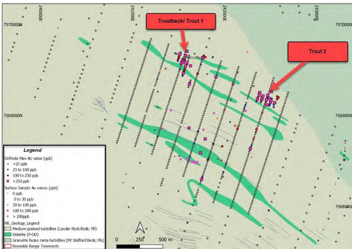
Figure 9. Map of Troutbeck (Trout 1&2) Prospect with drillhole and surface Au values overlying local geology.
