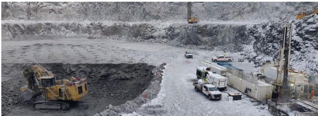
*Figure 3 - Sable open pit operation (left) and the completed reverse circulation drilling program (right). A similar set-up will occur next week for the commencement of the delineation and geotechnical Sable underground drill program.*
