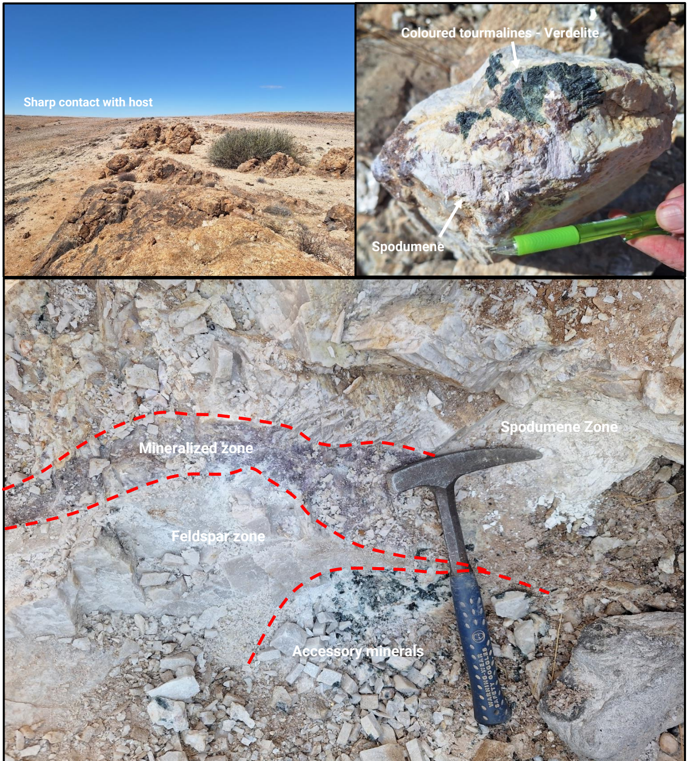
Figure 3 - Field photos of the Kestrel pegmatite illustrating mineralized zonation and different typical LCT mineral types
