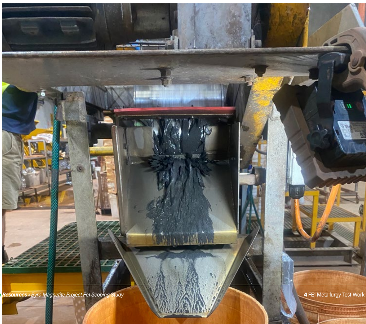
Figure 4-1: Wet LIMS Laboratory Unit at IOTC Recovering Magnetite Concentrate.
