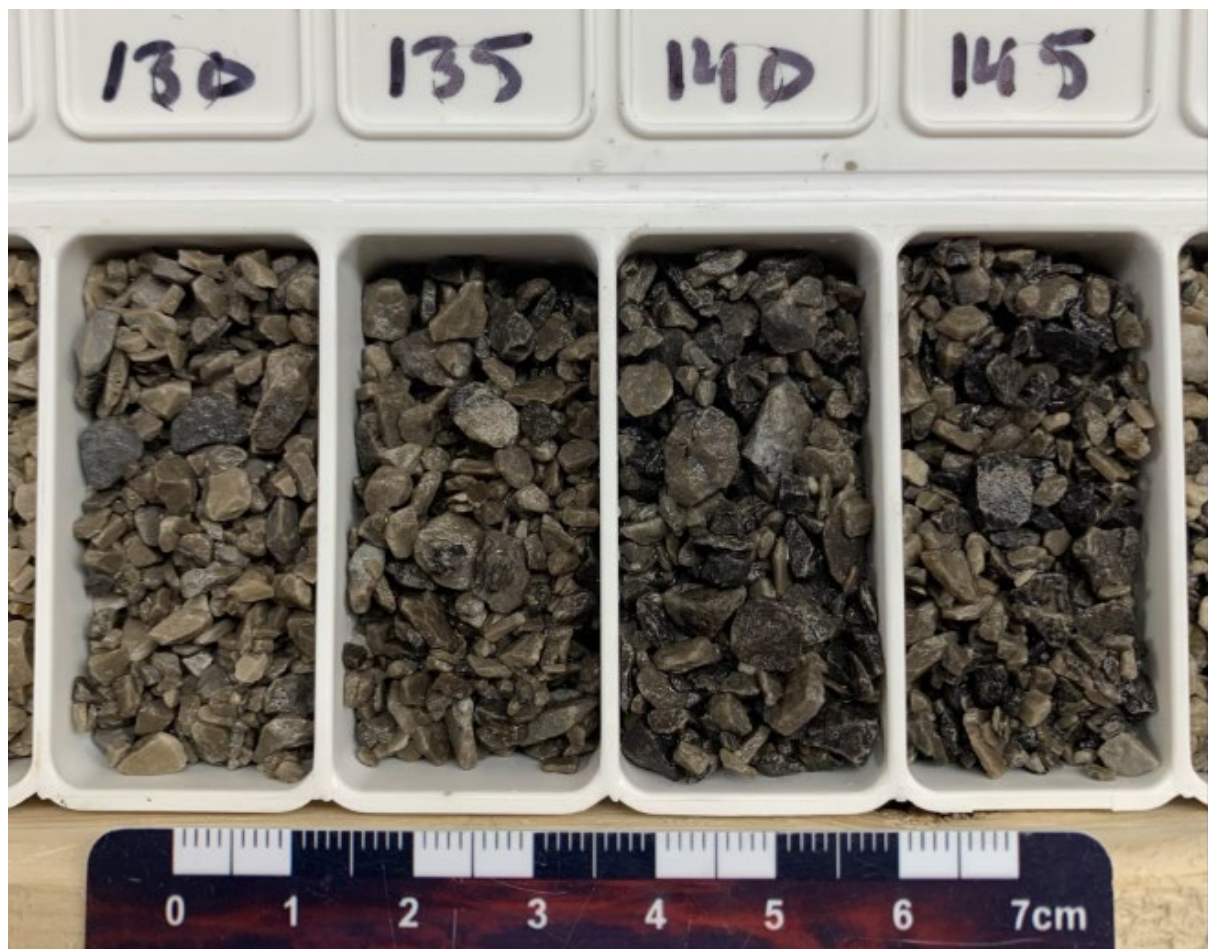
Figure 3: RC Drill chips from drill hole SR24-03 from the Gap Prospect. The interval is from 130ft (39.6m) to 145ft (44.2m) downhole. Chalcocite (80% copper) veins and chips are visible as dark grey.
