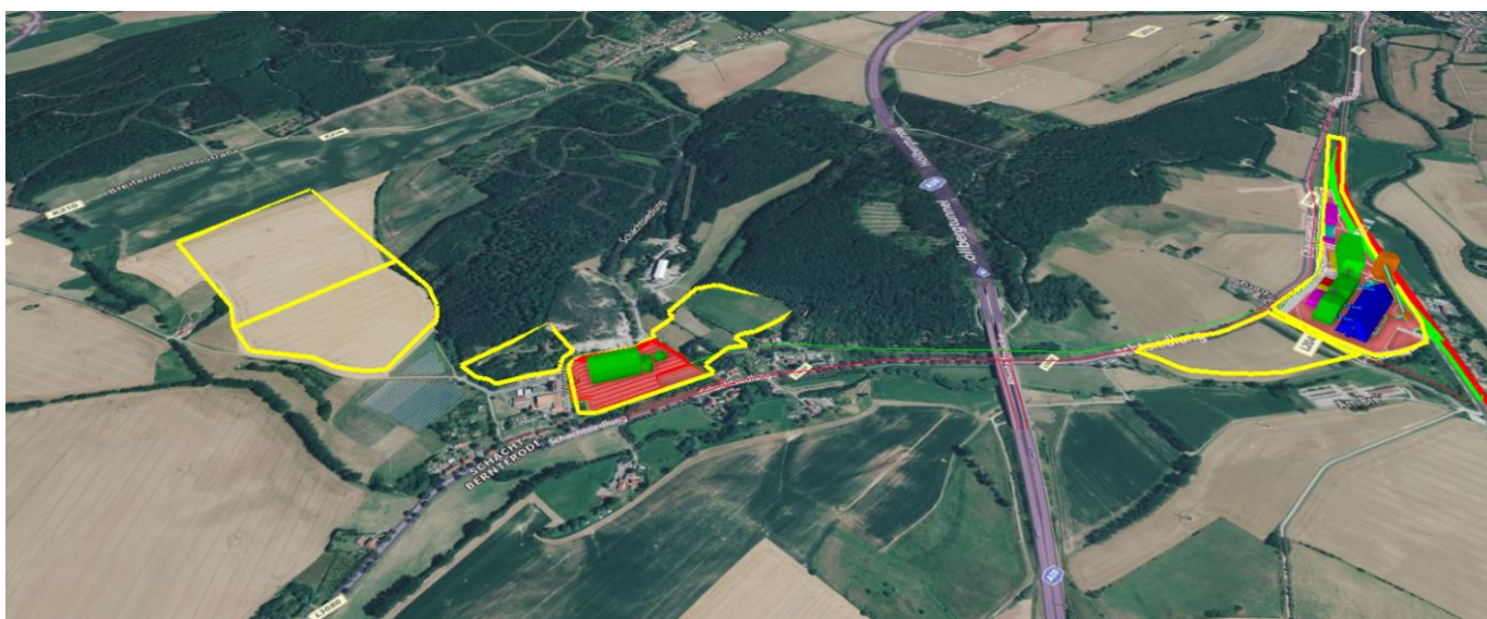
Figure 3: 3D renderings of Ohmgebirge surface development under PFS design; blank yellow outlines highlight previous footprint no longer required for shaft headframe and infrastructure, raw ore stockpiles and interim tails stockpiles
