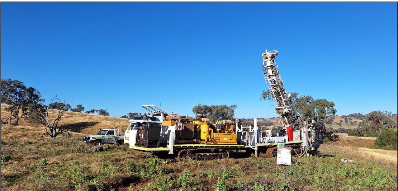
Figure 1: RC drill rig collaring hole SPRC001/Site SP016 at the Spur Prospect
