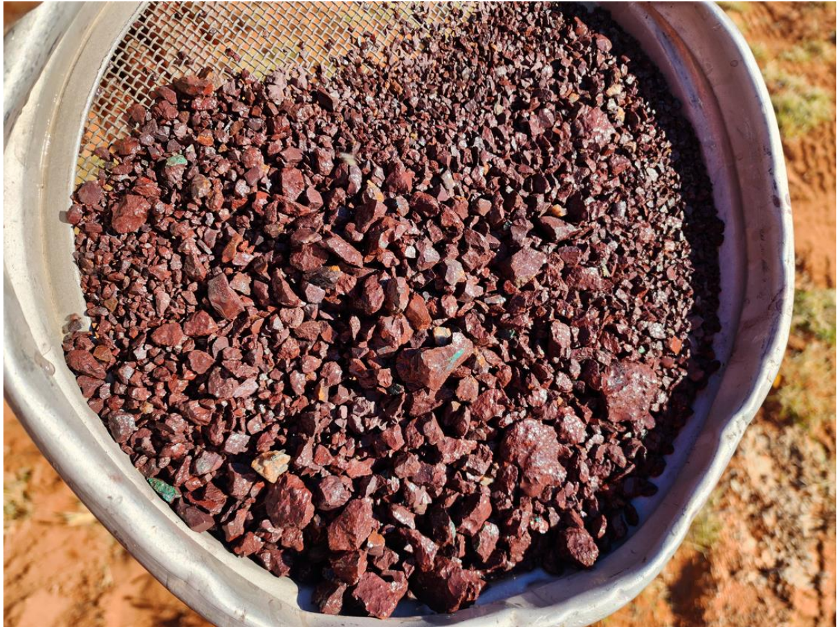
Figure 3: Mineralisation intercepted at the K vein prospect with visible malachite and strong haematite alteration.
