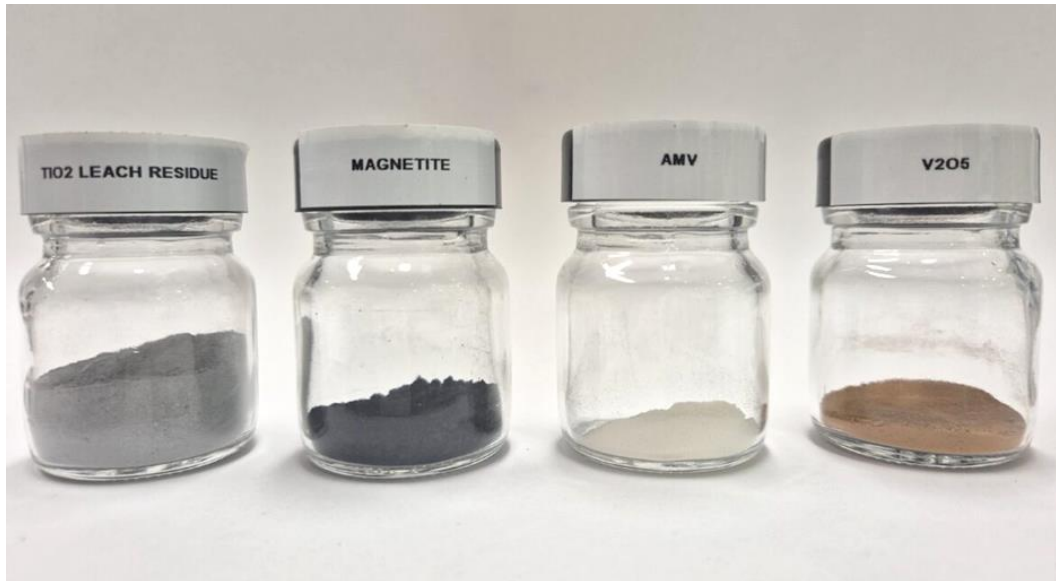
Image 1: Samples - titanium dioxide (leach trials), magnetite (iron recovery trials), “AMV” (ammonium metavanadate is a pre-cursor to V 2 O 5 preparation) and vanadium pentoxide (vanadium recovery trials) (source: CSIRO)
