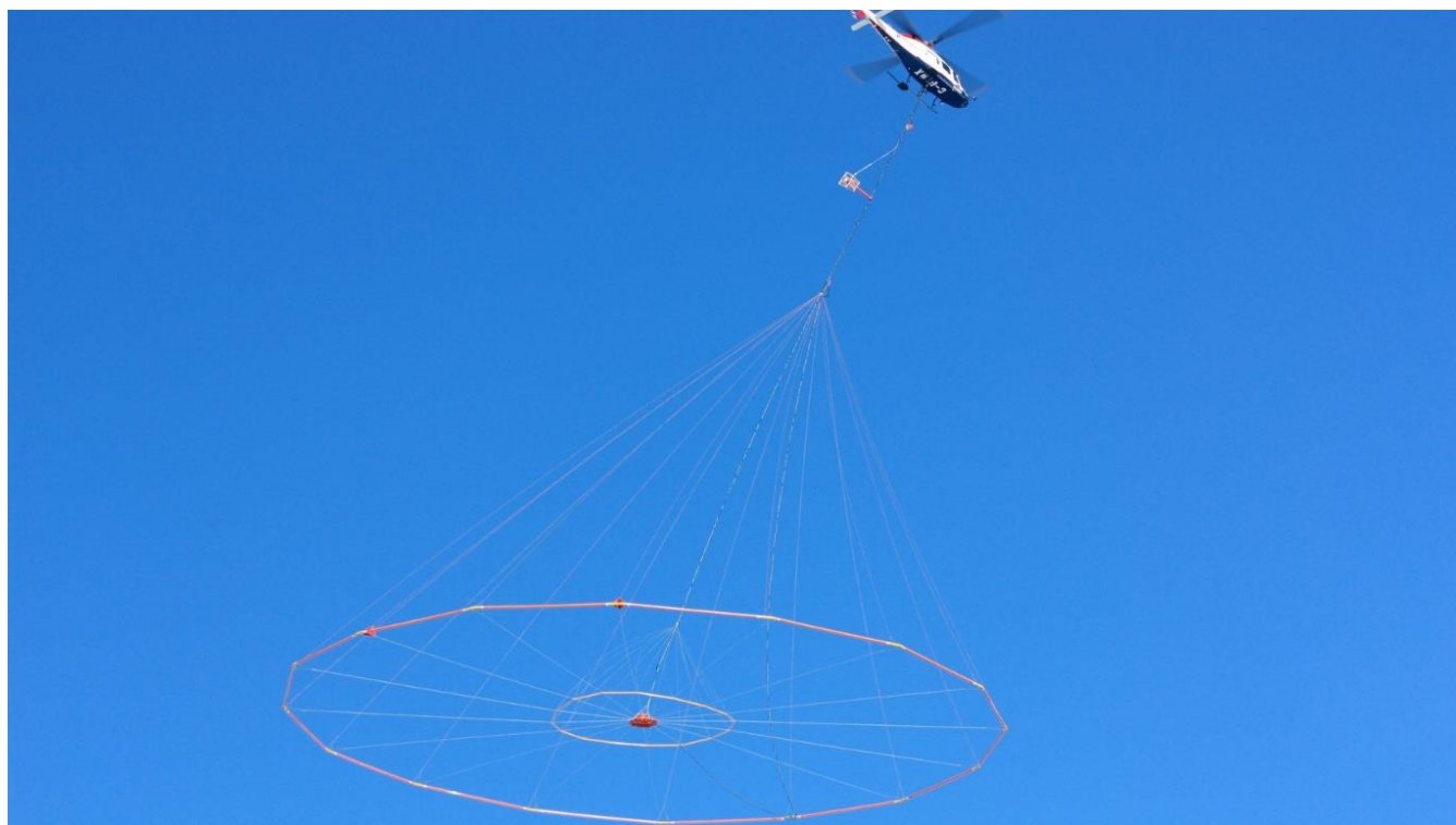
Figure 3: Helicopter Borne VTEM™ array
