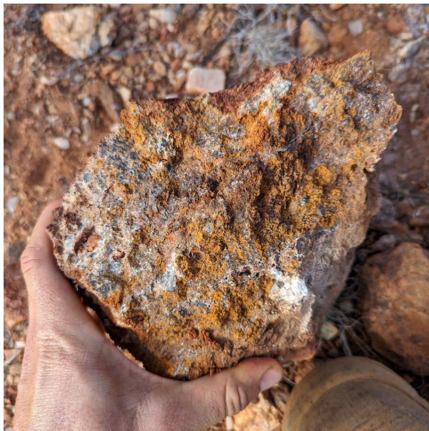
Figure 1: Photo of zinc-rich siliceous gossan sample TIG013B from Tiger which returned 27.1% Zinc in addition to 1.4% Cu, 60.1g/t Ag and 0.3g/t Au.
