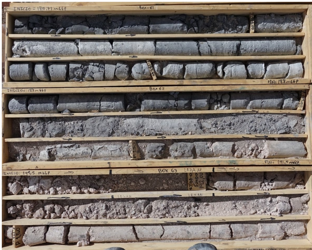
Figure 6: Unit 4 polymict reworked volcanic unit, beneath the salar and lava flows to the west.
