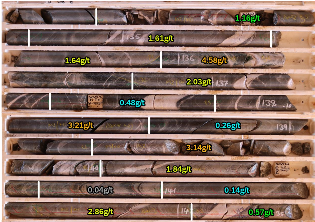
Figure 5. – Core showing the extensional footwall veining (Flats) from 134.2m in GC4523 which graded 6.4m at 1.95g/t.
