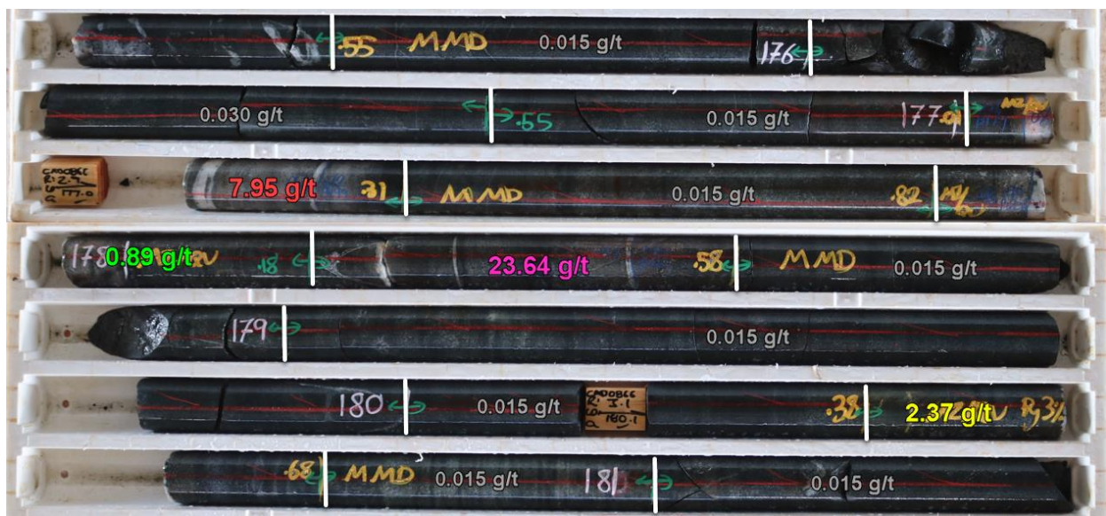
Figure 9. Core showing flat stacked extensional veining from Oval Fault footwall, from 177.0m in CAD0866 which graded 6.0m at 2.41g/t.
