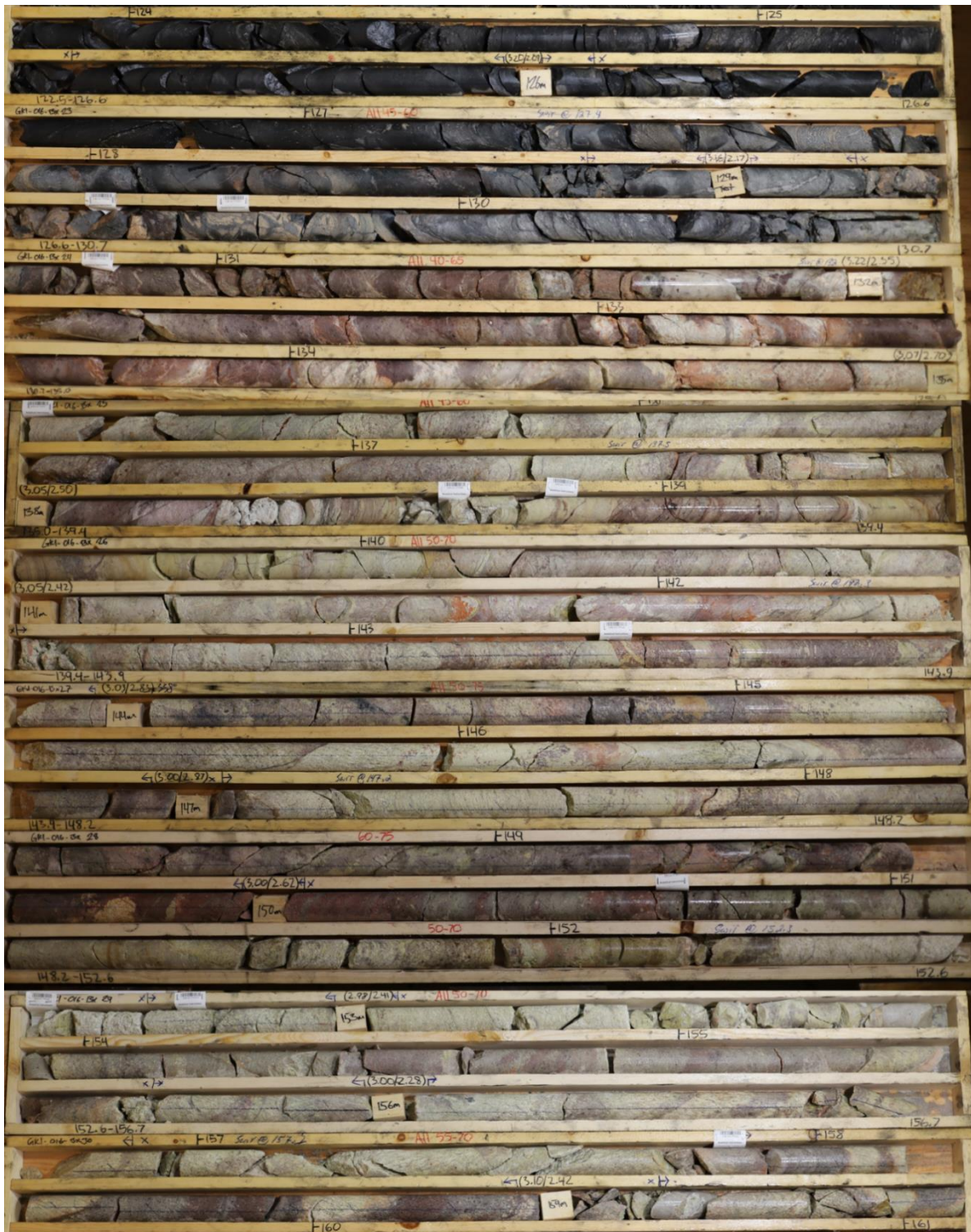
Figure 4: Core photographs showing redox alteration front in GKI-016.
