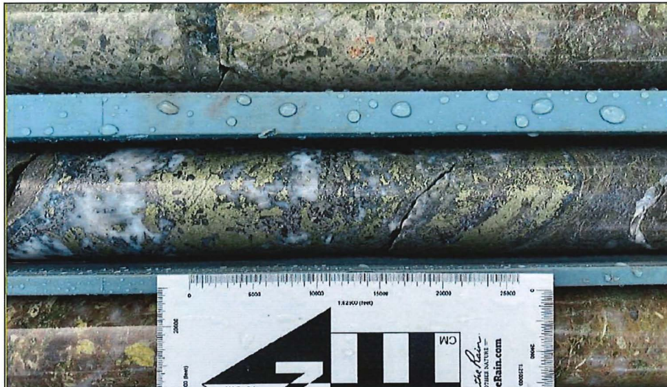
Figure 2.8: Mineralisation in veins of altered granite porphyry chalcopyrite, arsenopyrite, pyrite and galena in drill hole 22NGD108
