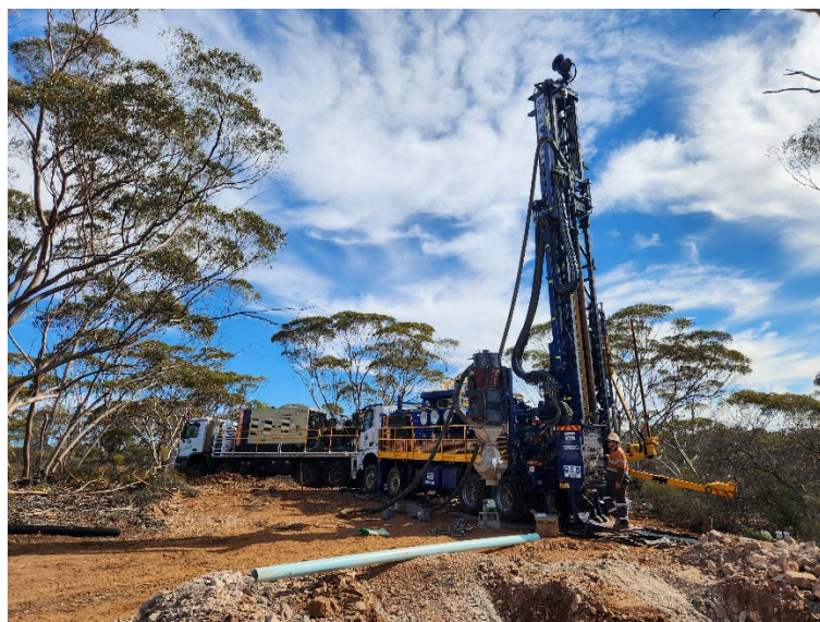
Figure 1: RC rig drilling targeted step-out north-easterly extension of Big Red pegmatite
