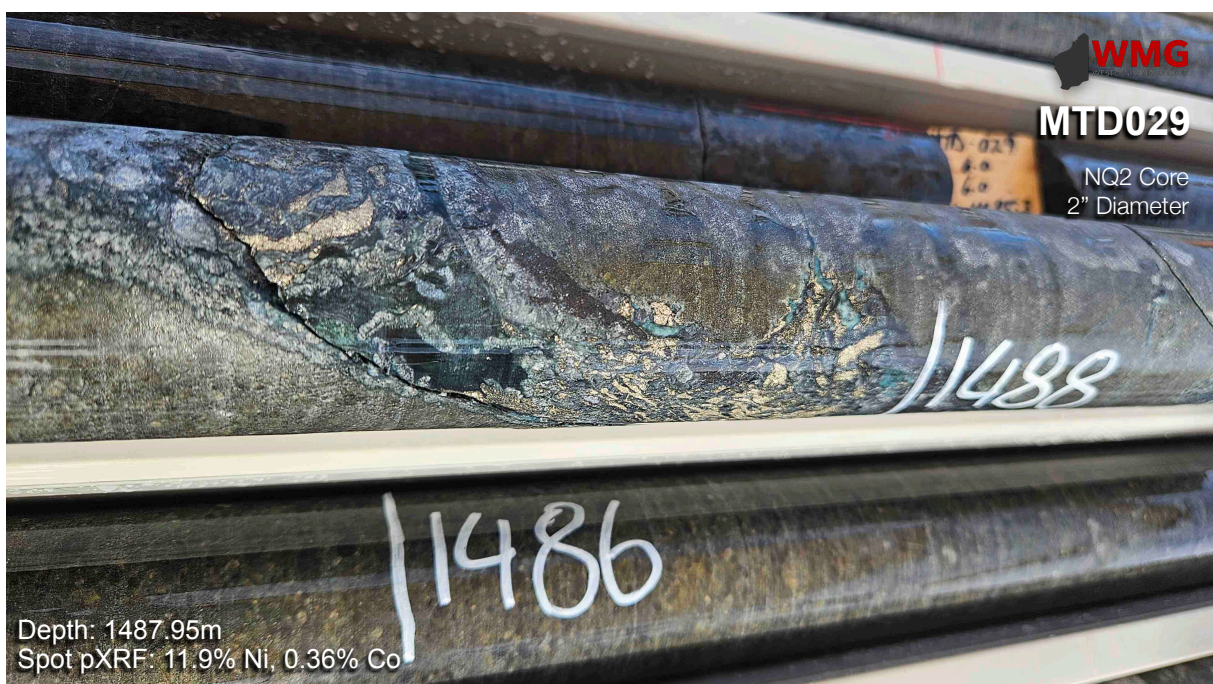
Figure 2: Photos showing examples of sulphide segregations and veinlets in hole MTD029 (EIS3) Note: core is NQ2 being 2 inches or 50mm diameter
