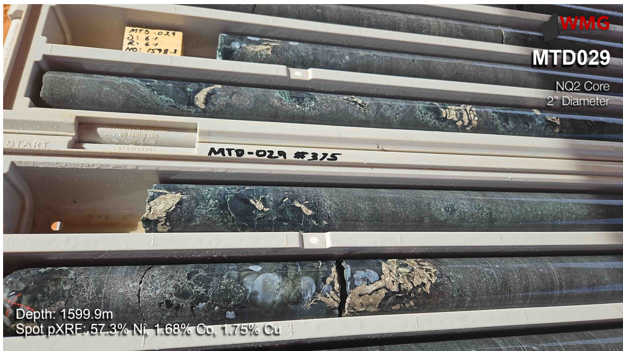
Figure 1: Photos showing examples of large sulphide segregations in hole MTD029 (EIS3) Note: core is NQ2 being 2 inches or 50mm diameter
