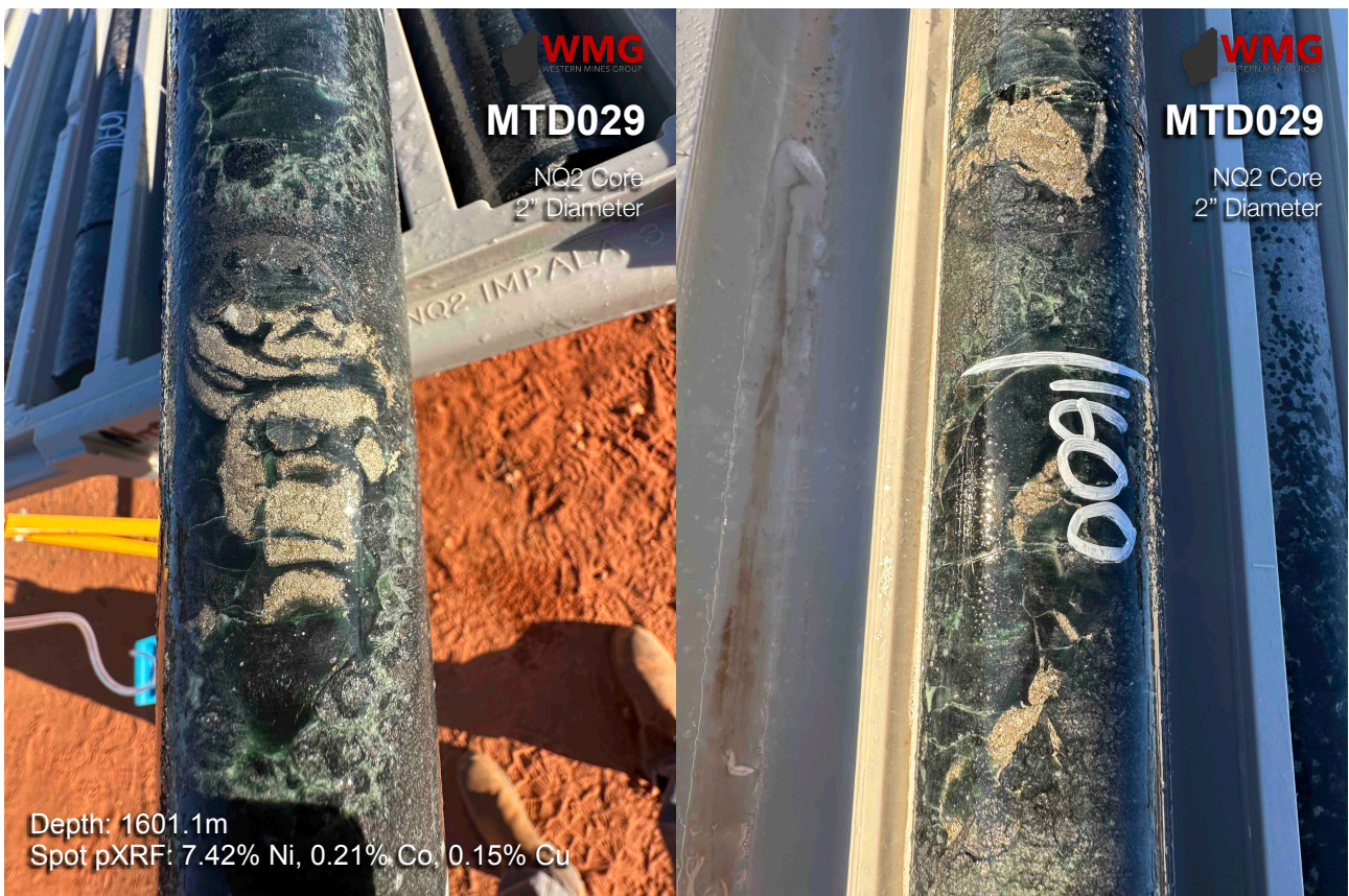
Figure 4: Photos showing examples of large sulphide segregations in hole MTD029 (EIS3) Note: core is NQ2 being 2 inches or 50mm diameter
