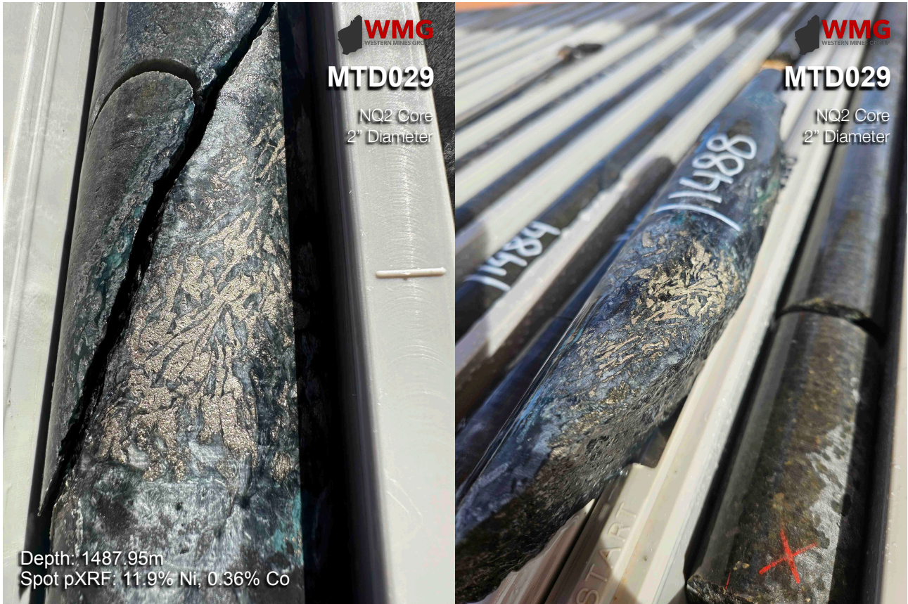
Figure 3: Photos showing examples of sulphide segregations and veinlets in hole MTD029 (EIS3) Note: core is NQ2 being 2 inches or 50mm diameter
