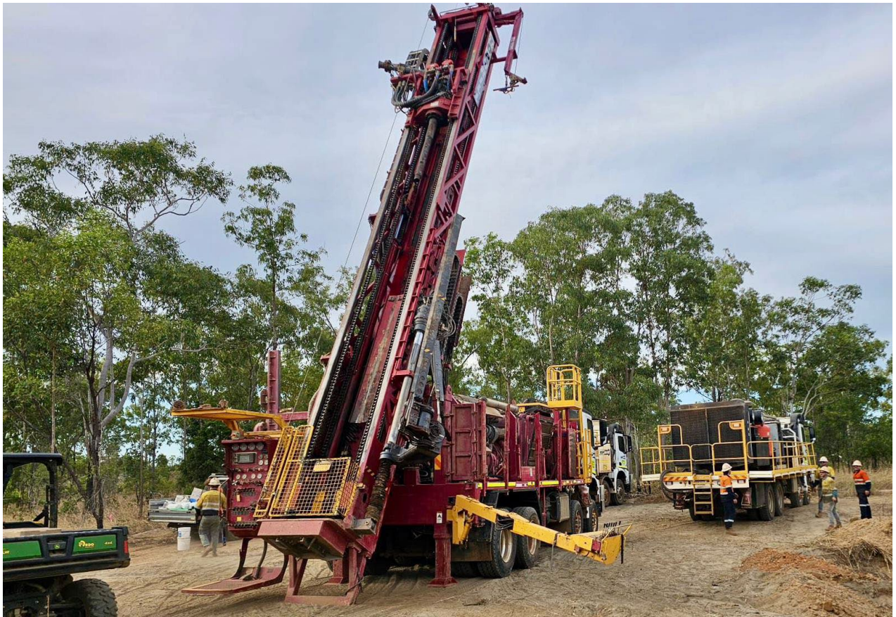
Figure 1: RC drilling underway at Nabarlek Uranium Project, Northern Territory.
