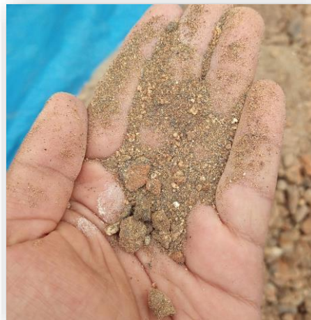
Figure 3: Rock sample CJV-001 (247ppm Li, 695ppm Rb, 108ppm Cs)
