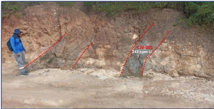
Figure 3: Rock sample CJV-001 (247ppm Li, 695ppm Rb, 108ppm Cs)
