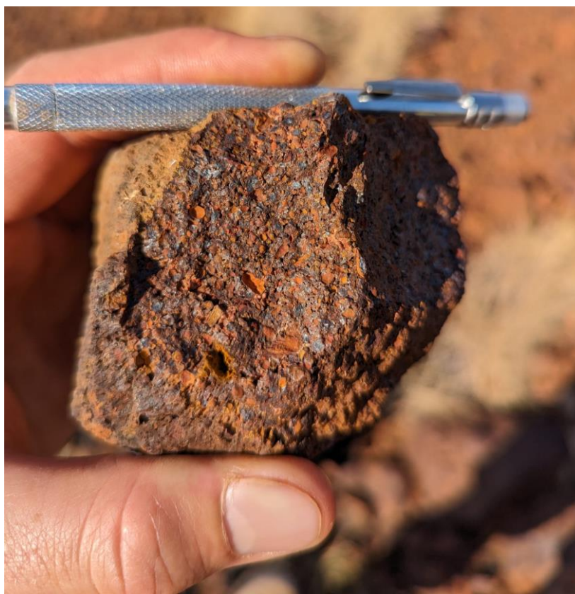
Figure 3: Robe River pisolite hand sample located from Mesa 3 (200m west of tenement boundary) showing representative Robe River pisolite found on Mesa 1 and Mesa 2.
