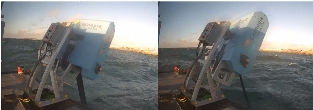
Module reorienting automatically to maintain alignment of drum and belt
