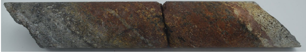
Figure 4: Hydrothermal hematite, argillization, and uraninite blebs at 419.7 m with a maximum of 7,500 cps
