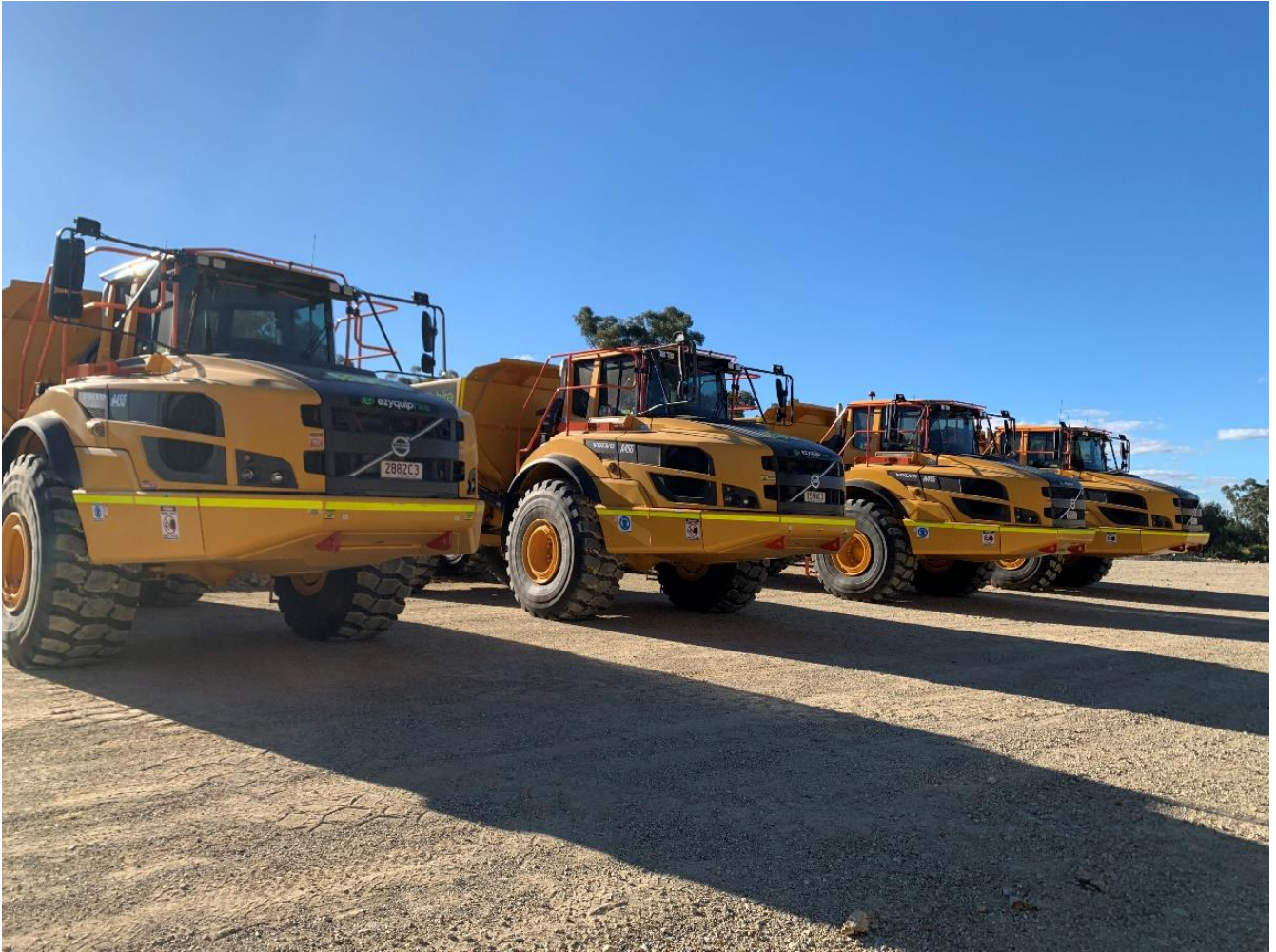
Figure 4: Open pit fleet mobilisation – a new mining fleet has been mobilised to site which includes 6 x 45 tonne trucks, 1 x 50 tonne excavator and 1 x 90 tonne excavator, 1 x D9 Dozer
