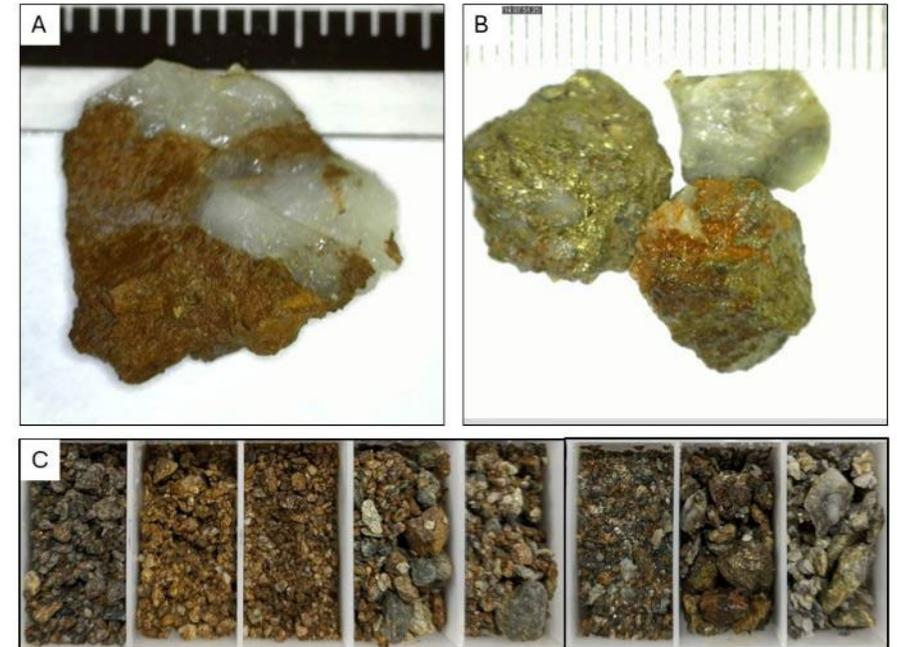
(A) RC ROCK CHIP SHOWING BROWN EUHEDRAL ANKERITE AND QUARTZ FROM CRC0012; (B) RC ROCK CHIPS SHOWING QUARTZ VEINS WITH VISIBLE CHALCOPYRITE FROM CRC0037, and (C) EACH SAMPLE REPRESENTS 1M OF RC CHIPS FROM 2M –9M DEPTH FROM CRC0037. NOTE THE HIGHLY OXIDIZED AND SULPHIDE RICH MATERIAL AS WELL AS ABUNDANT QUARTZ.
