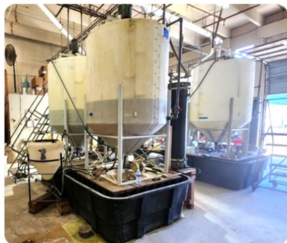
Figure 2 – PMR Pilot Plant Reagent Mixing/Recovery Circuits
