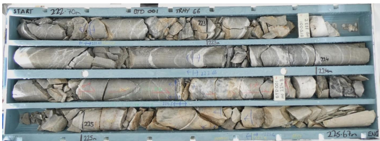
Figure 4: BTD001 from 220.03 m – 225.67 m. Leven Star hanging wall splay structure returning 5.60 m @ 3.14 g/t Au from 219.8 m (including 3.04 m @ 4.97 g/t Au from 222.36 m).
