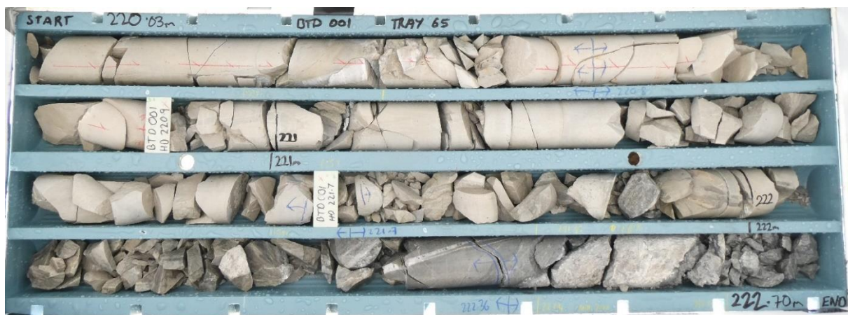
Figure 3: BTD001 from 276.26 m – 279.13 m. Structural repeat (or overlap) of Leven Star Reef at depth returning 4.25 m @ 5.88 g/t Au from 274.75 m (including 2 m @ 11.15 g/t Au from 277 m).
