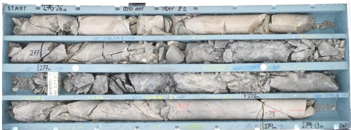
Figure 3: BTD001 from 276.26 m – 279.13 m. Structural repeat (or overlap) of Leven Star Reef at depth returning 4.25 m @ 5.88 g/t Au from 274.75 m (including 2 m @ 11.15 g/t Au from 277 m).
