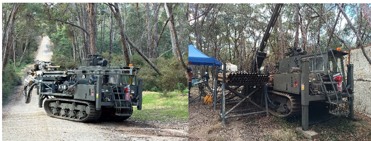
Photos of the diamond drill rig used in the program and a typical drill site.
