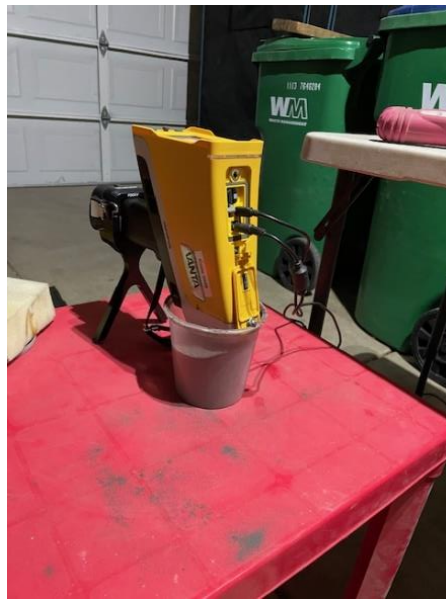
Figure 2 Once crushed, samples were rechecked with both a magnetic susceptibility meter and a pXRF analyser to ensure the correct mixing ratios were used to achieve the sought after long term run of mine grade.
