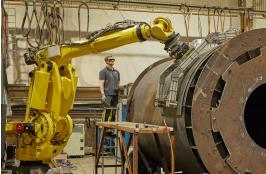
Figure 2: Robotic Laser Welding & End-cap Jig illustrating layering of carbon steel plate
