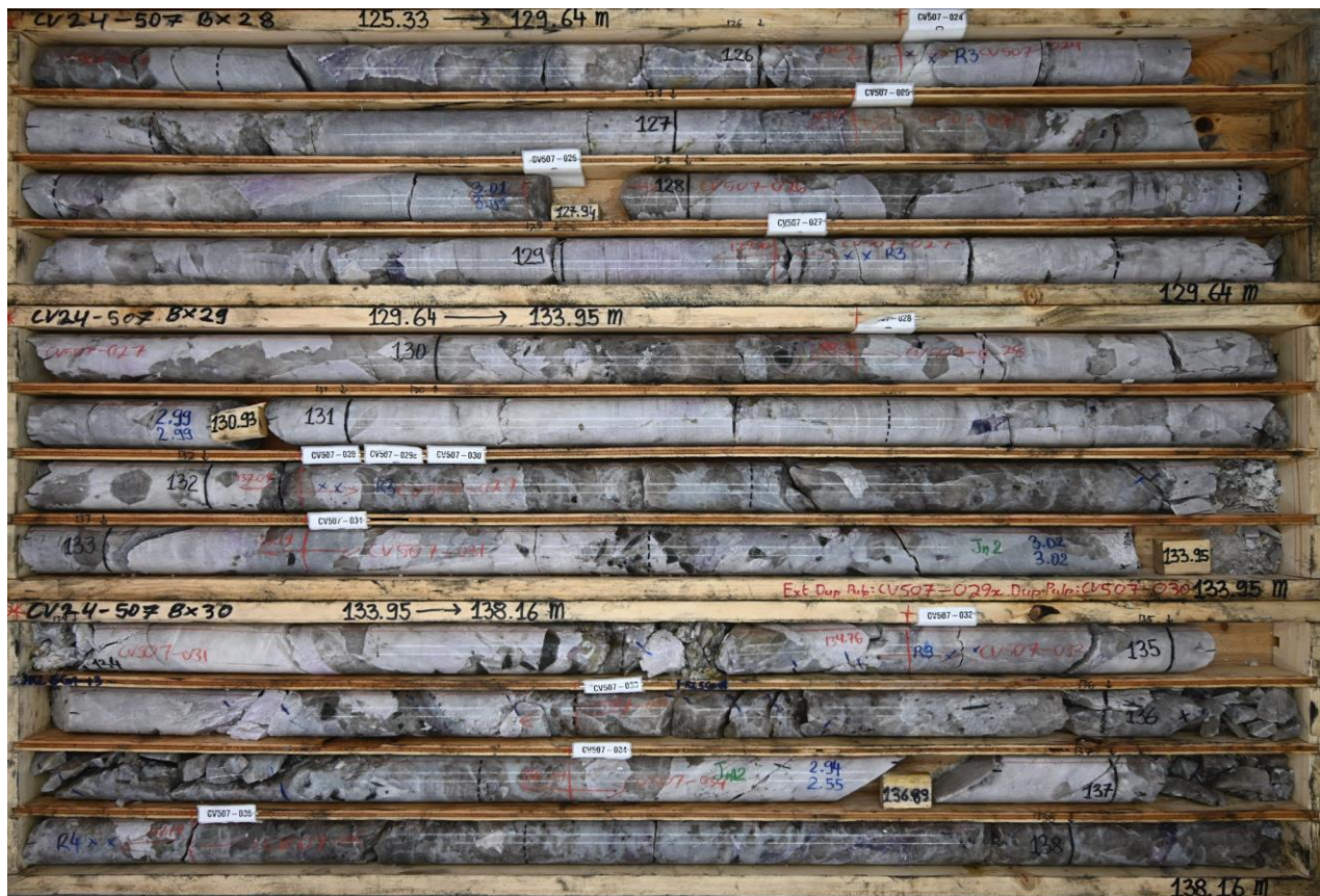
Figure 3: High-grade spodumene pegmatite drill intercept from the Vega Zone at CV13 (drill hole CV24-507), averaging approximately 3.5% \text{Li}_2\text{O} over interval presented (125.3 m to 138.2 m), including 1.7 m at 7.01% \text{Li}_2\text{O} – the highest grading individual core sample reported to date from Corvette.
