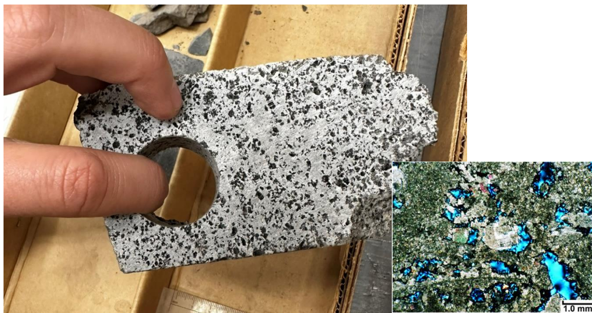
Figure 1: Core from the Lisbon D-616 well (8,619' depth) showing exceptional dolomitic vuggy porosity. Note core plug sample (circular hole). Semi-inset: Thin section at 8,619' showing a 100% dolomite reservoir, with secondary porosity enhanced by hydrothermal dolomitization (pore spaces in blue)
