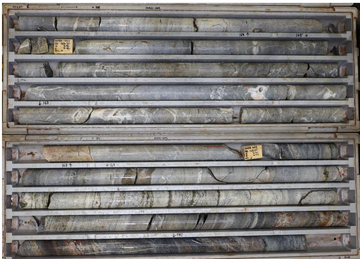
Figure 5. Example of interpreted high-sulphidation epithermal alteration zone in OND003 containing vein sulphides with phyllic alteration, extending from the high-grade silver mineralisation from approximately 158m – 184m.
