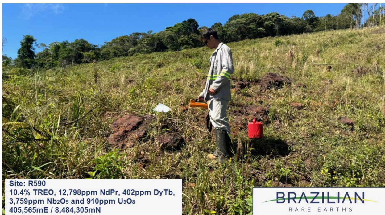
Figure 7: Pelé Target 1 - Outcrop sample R590 with REE-Nb-Sc-U mineralisation
