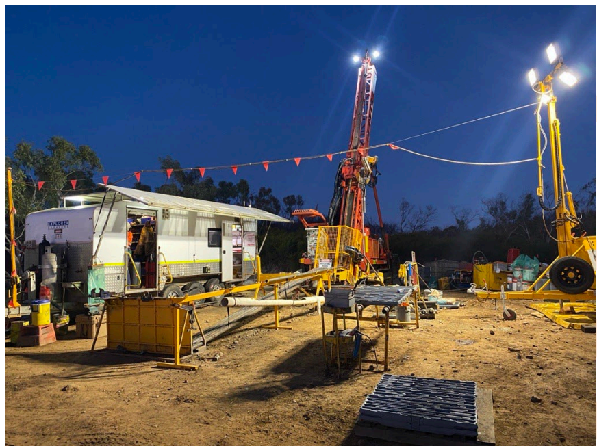
Figure 1. Diamond Drill Rig at Hardway
