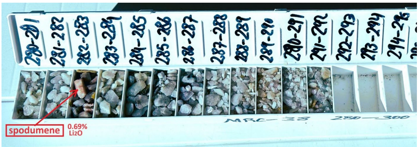
Figure 3: Part of the 280m-300m chip tray of MRC 38, displaying mineralisation & grade.
