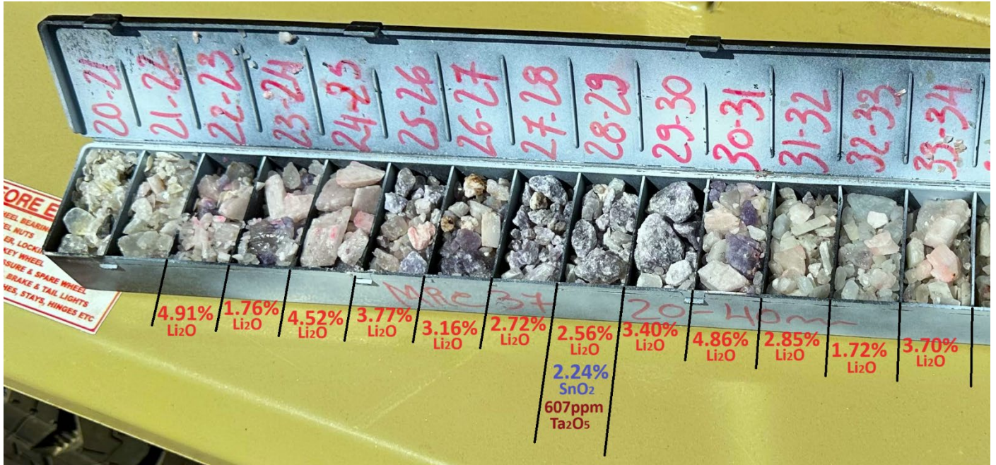
Figure 2: Part of the 20m-40m chip tray of MRC 37, displaying mineralisation grades.
