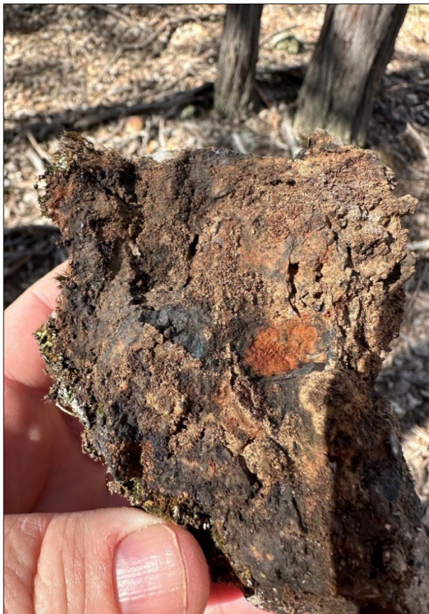
Figure 2 – Silver-Base metal mineralisation within ferruginous gossan yielding 87.8 g/t Ag , 1.5% Cu-Pb-Zn & >1% Ba from sample 3000728
