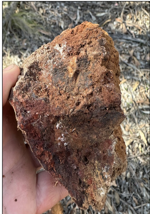
Figure 3 – Silver-Base metal mineralisation within gossan yielding 36.8 g/t Ag , 0.3% Cu-Pb-Zn & 0.2% Ba from sample 3000766
