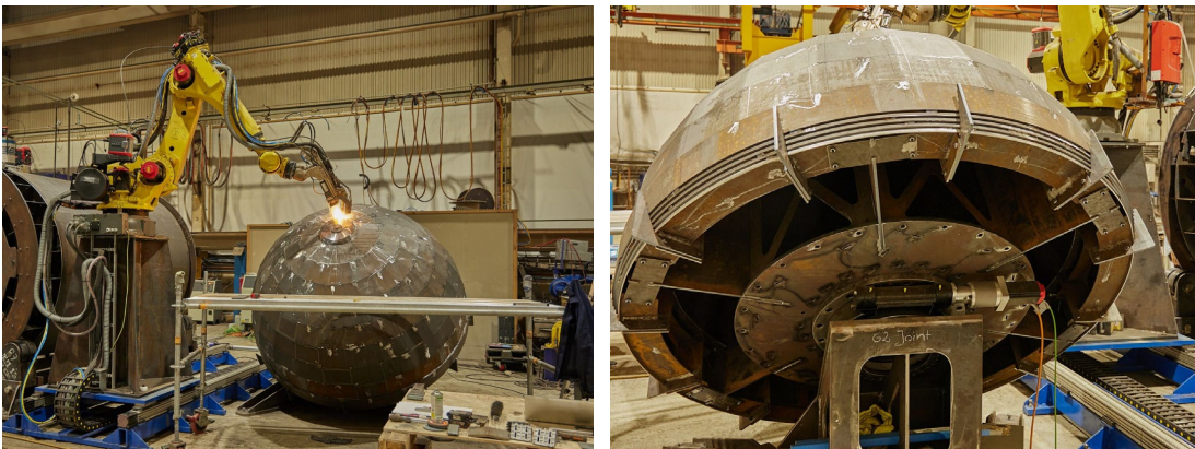
Figure 2: Robotic Laser Welding & End-cap Jig illustrating layering of carbon steel plate
