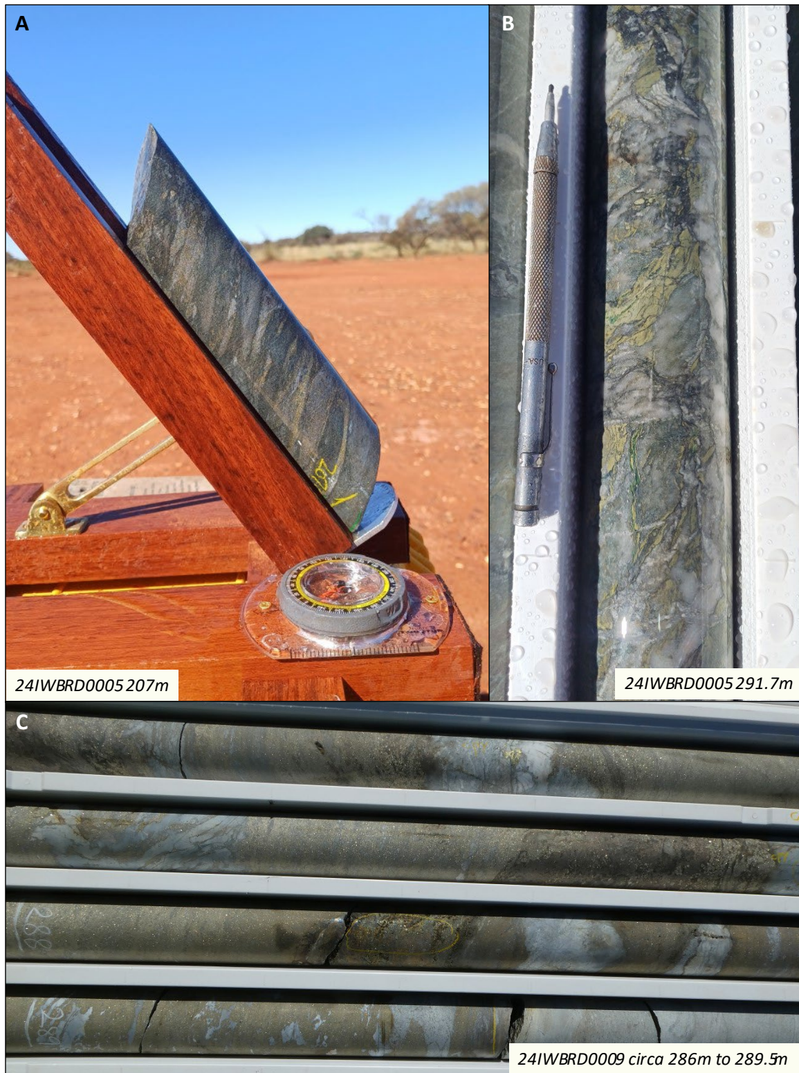
Figure 7: A. An example of an altered shear zone within NQ2 core 24IWBRD0005. B. An example of a deformed and altered early quartz veining within NQ2 core from 24IWBRD0005. C An example of massive to semi-massive sulphide (pyrite dominant) intercalated with narrow quartz veins and/or micro-crystalline chert within NQ2 core from 24IWBRD0009.
