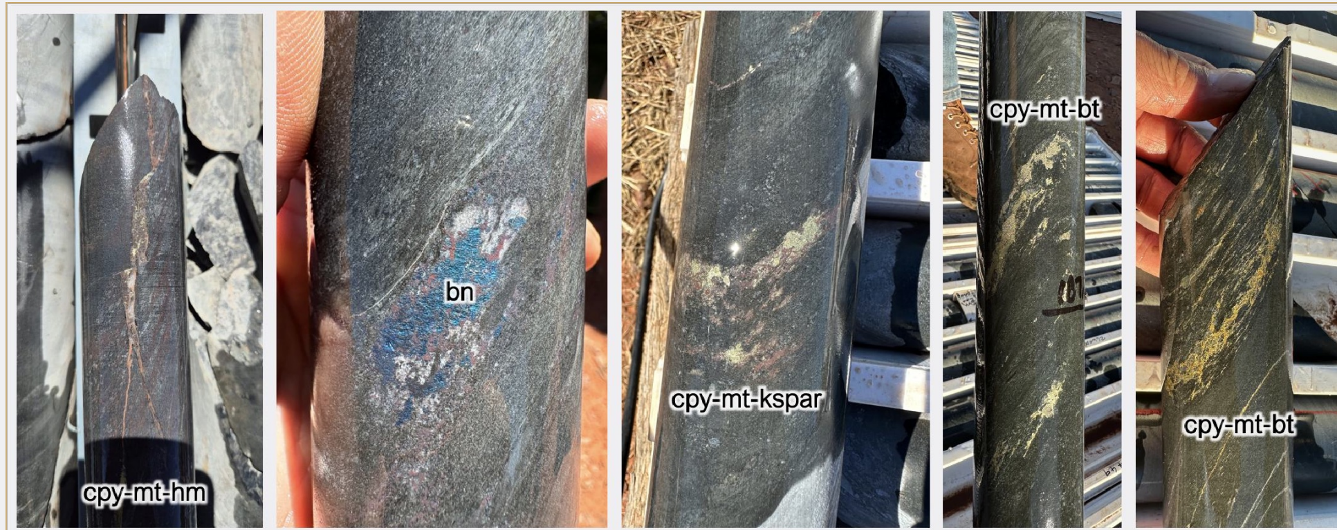
Observations from hole 24WADD002 drill core showing IOCG-style mineralisation including magnetite +/- hematite (mt, hm), bornite (bn), chalcopyrite (cpy), potassic feldspar (kspar) and biotite (bt). Visible gold was also observed. 4
