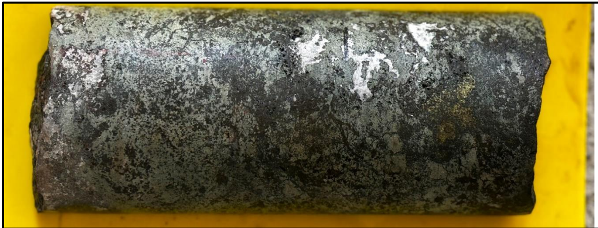
Figure 5 Drill core from 393.5m in ZRSD24148, assaying 4.0g/t Au Eq (0.3g/t Au, 0.2% Cu, 6.2% Zn and 6.1g/t Ag)
