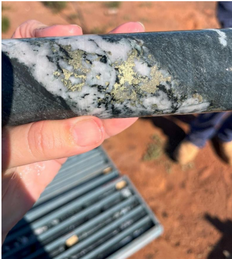
Figure 2 – Example of a mineralised quartz vein containing chalcopyrite and pyrite mineralisation at 301.4m depth in CBLRCDD065. Vein is approximately 5cm wide.
