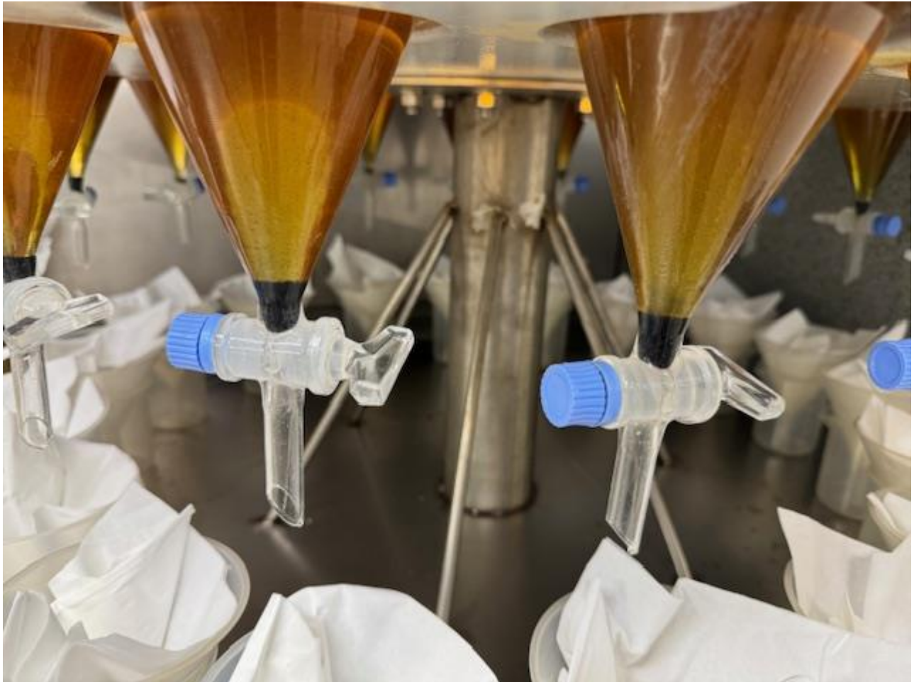
Figure 2: Capel samples undergoing float/sink analysis with T.B.E at Diamantina
