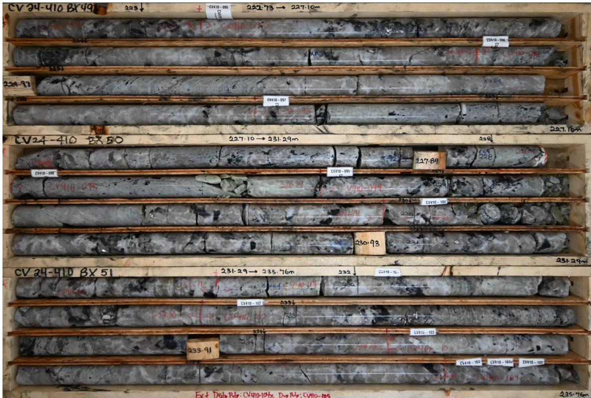
Figure 4: Spodumene pegmatite in CV24-410. Core grades 5.24% \text{Li}_2\text{O} over 2.2 m (226.5 m to 228.7 m).
