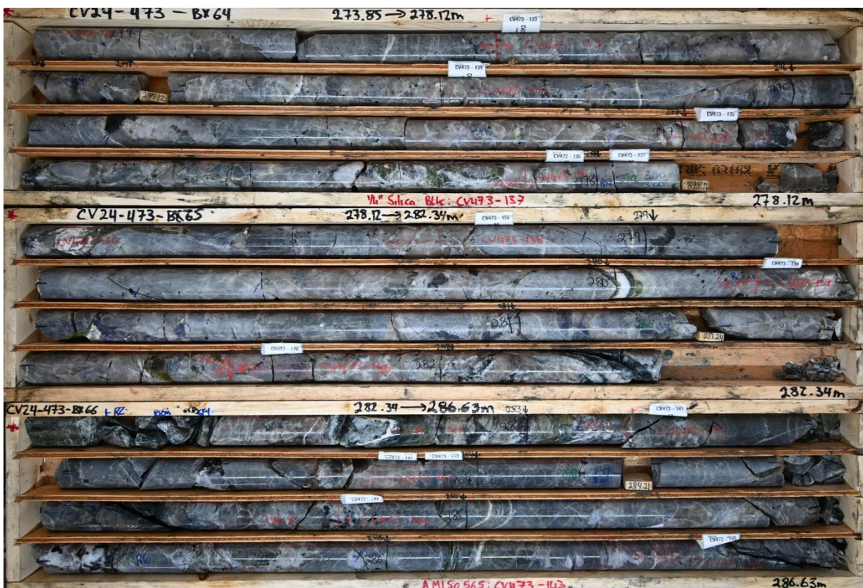
Figure 2: Spodumene pegmatite in CV24-473. Core grades ~4% \text{Li}_2\text{O} over interval.
