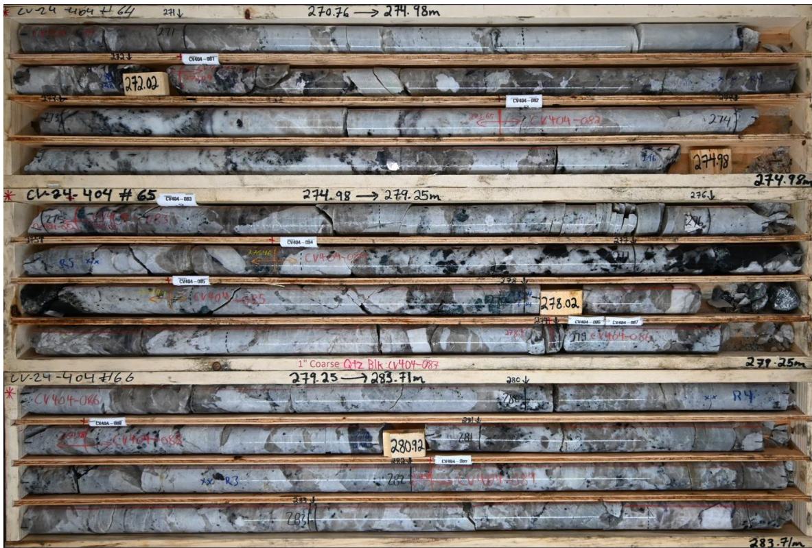
Figure 3: Spodumene pegmatite in CV24-404. Core grades ~3.7% \text{Li}_2\text{O} over interval.
