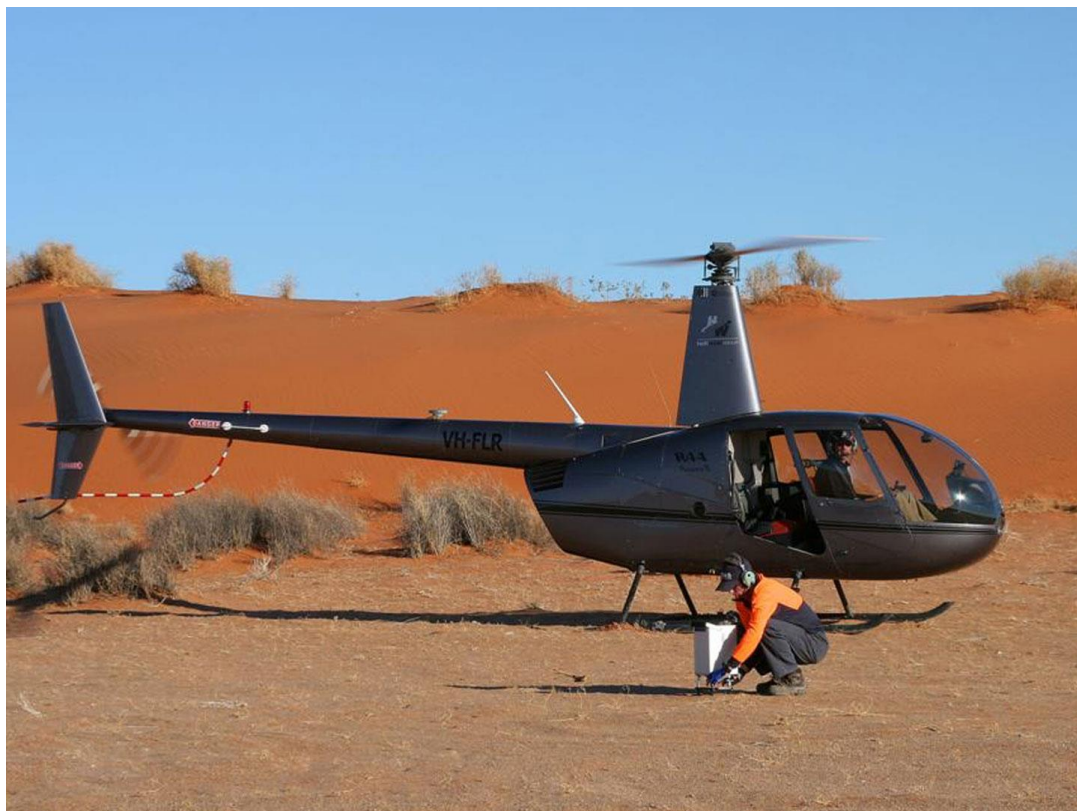
Figure 1 Helicopter-assisted ground gravity survey station (Atlas Geophysics)
