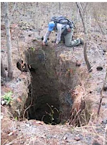
Figure 3: A photo of a 3.5 m deep prospecting trench and brecciated altered pyroxenite
