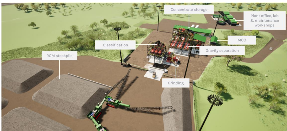
Figure 11 Process Plant Layout
