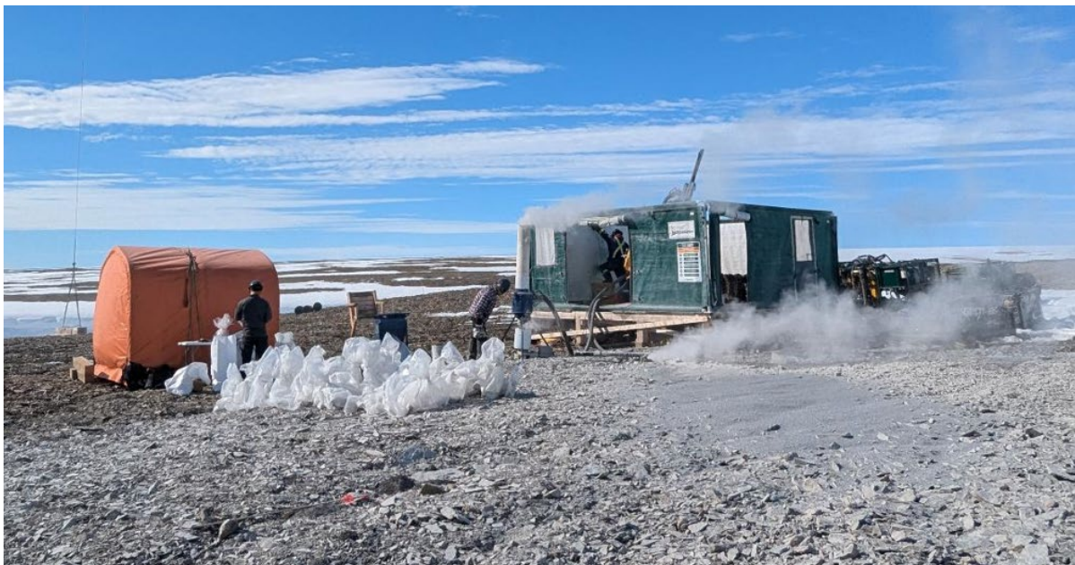
Figure 1: Reverse Circulation (RC) drilling underway at the Chinook Deposit, Storm Project, Nunavut.
