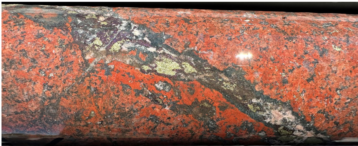
Figure 6. Carbonate-bornite (purple)-chalcopyrite (yellow)-specular hematite (dark grey) vein and disseminated chalcopyrite and bornite (purple) from 1074m - 1074.15m
