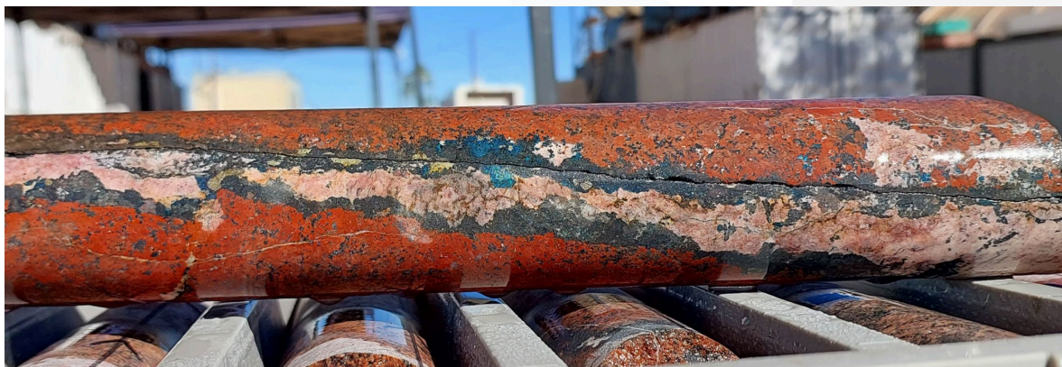
Figure 7. Carbonate vein with outer vein and disseminated bornite (blue) and specular hematite (dark grey) from 1081.2m - 1081.5m.
