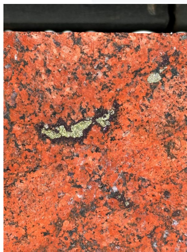
Figure 4. Disseminated chalcopryrite (yellow) mineralisation surrounded by (rimmed) by high tenor copper species bornite (purple) from 1070m - 1070.2m.
