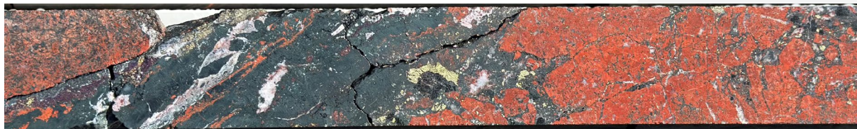
Figure 3. Chlorite carbonate breccia with clast and vein bornite (purple) and chalcopryrite (yellow) from 1065m - 1065.4m.
