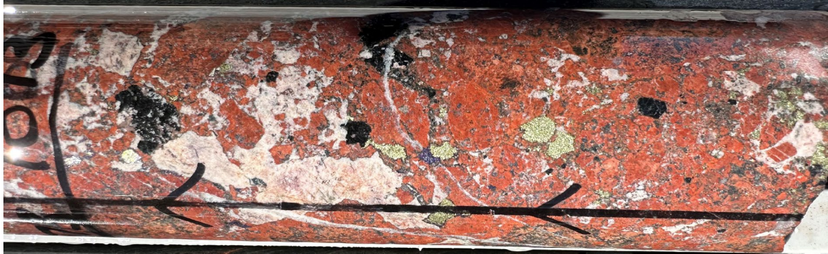
Figure 5. Carbonate breccia with clasts of chalcopyrite (yellow) and bornite (purple) in intense k feldspar - hematite altered granite from 1072.8m - 1073m.
