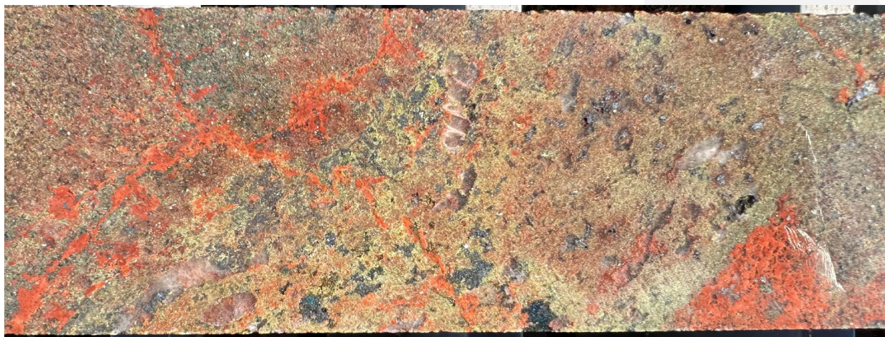
Figure 8. WBDD001 Wimberu granite with strong halo style sericite-specular hematite alteration and trace bornite (blue) from 319.6m - 319.7m assaying 0.12%Cu.
