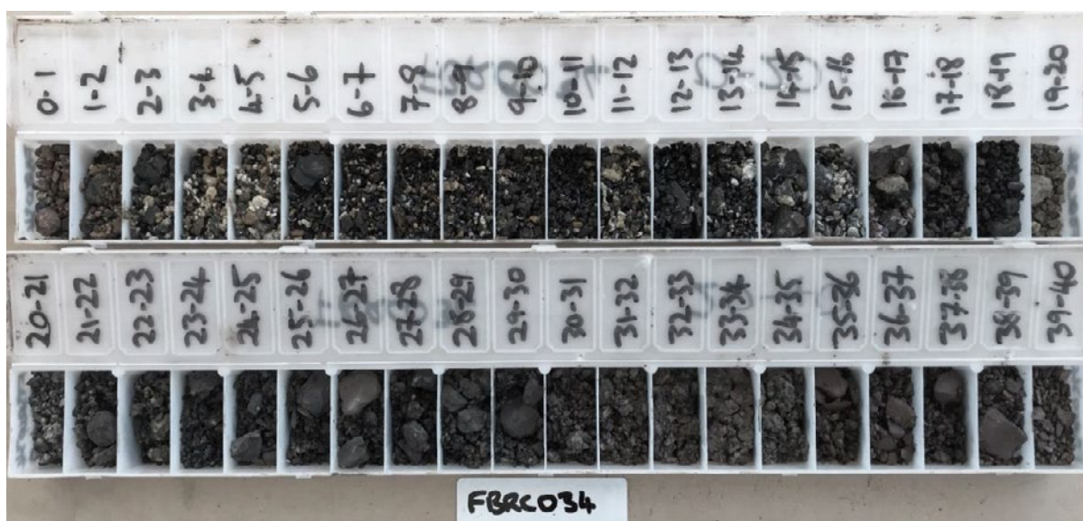
Figure 7. RC drill chip tray from LR1 (FBRC034 - 23m @ 11.5% Mn and 8.9% Fe from 5m)
