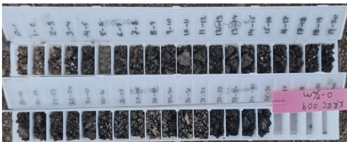
Figure 8. RC drill chip tray from KR1 (KKRC009 - 27m @ 11.8% Mn and 8.5% Fe from 4m)
