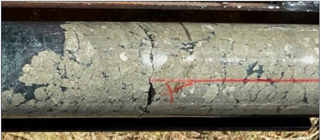
Figure 4: RMD001 massive pyrite, at 316m down hole. (See Table 2)
