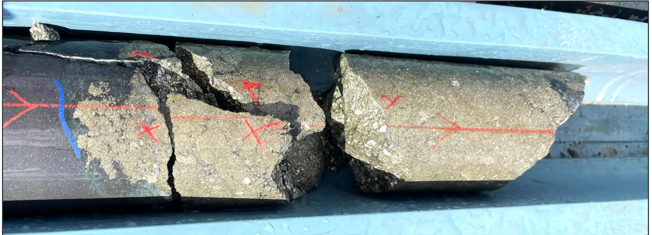
Figure 3: RMD001 massive pyrite, at 212m down hole. (see Table2)
