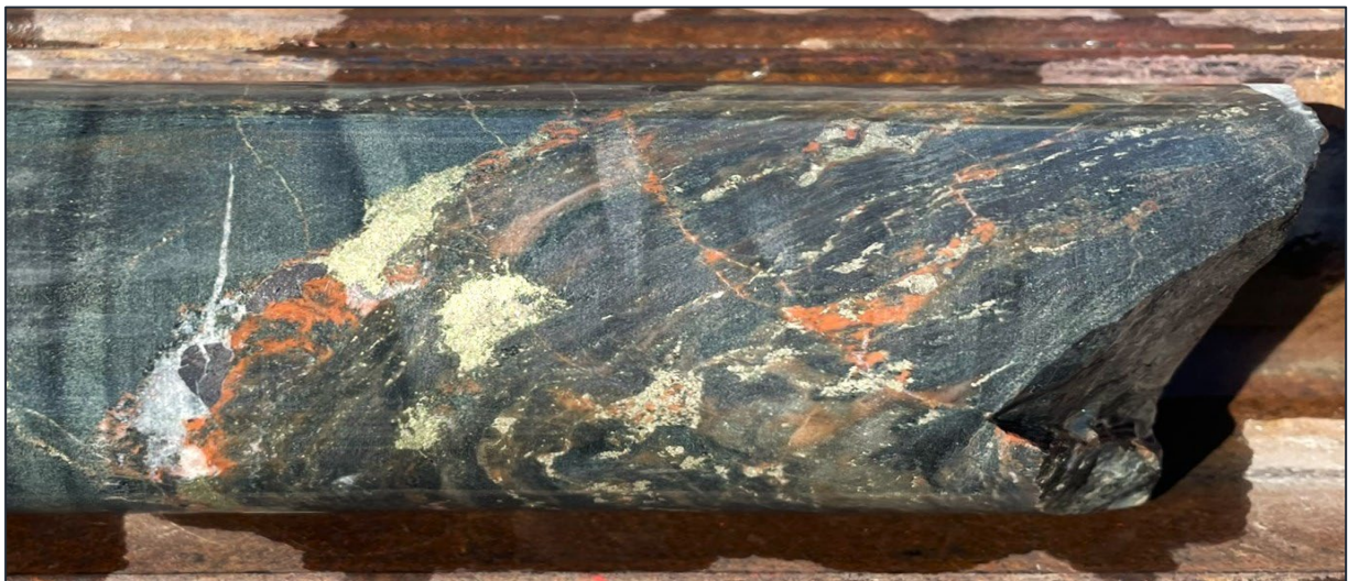
Figure 5: RMD001, showing a shear zone with magnetite, biotite, red rock, chalcopyrite and pyrite, at 306m down hole. (See Table 2)
